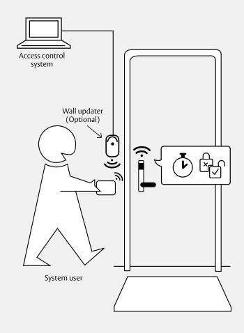
**Example:** Multiple door system securing a small medical centre. Low amount of changes on a daily basis but restricted time profiles are important.
